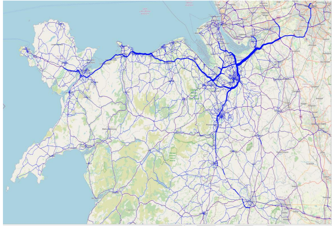
Figure - example of traffic flow comparison output from the North Wales Transport Model
