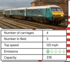
The Mark 3 carriages were developed as part of the InterCity 125 High Speed Train project in the 1970s. The loco-hauled Mark 3s have been used on "Gerald" Premier Service since 2008, providing a first-class service on the Cardiff-Holyhead route.
