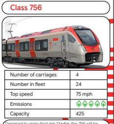
Designed by manufacturer Stadler, the 756 will be introduced on South Wales Metro services, providing major improvements in the customer experience from 2023. The Class 756s will be powered by overhead electric and batteries to Rhymney and Coryton, and by a diesel engine on the Vale of Glamorgan Line
