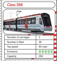
Stadler's CityLink tram-train forms the basis for the South Wales Metro Vehicles, which will enter service in 2022 on services to Merthyr Tydfil, Aberdare and Treherbert. These innovative vehicles, powered by overhead electric or batteries, are capable of running on traditional rail lines and light rail tramways.
